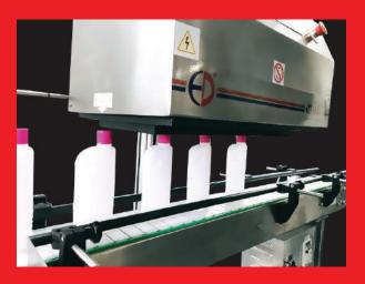
Once you have all information in place, you need to have an optimal sealing head and power supply. Tunnel coils are ideal for closures with smaller diameters. In the case of sports caps, deep tunnel coils are effective. Meanwhile, a flat coil is best suited for closures over 53 mm in diameter. However, a universal sealing head is the best option for application with a variety of closure sizes.
